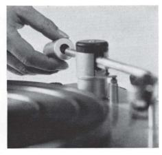
The head shell (16) is inserted at the front end of the tone arm and tightened by clockwise rotation of the nut (15). Upon insertion, the guide pin must be fitted into the groove of the pickup arm tube. The counterweight (13) is screwed onto the rear end of the tone arm with the small bore diameter looking forward.
