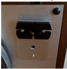
**Note**; If you want to route the wiring into the plinth. Feed through the slot in the Wand mount before adding screws. (But good to 'practice' other steps first)
