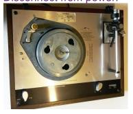
**Step 3**; Remove the arm cable clamp and the white cable cover.
