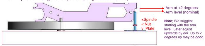
**Step 2**; Position the mount using the protractor (Slide back and forth)
