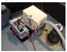
**Step 5**; Remove the lift mechanism and cable base (Four screws)
