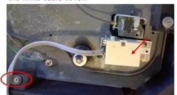
**Step 2**; Support the turntable upside down and remove the bottom cover.
