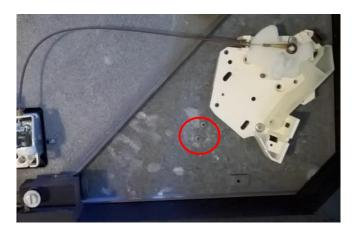
Hint; Improve your Thorens by adding damping material to the underside of the sheetmetal panels and the bottom cover while it is off. (but watch adding too much weight to the floating chassis part)
