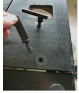
*Hint;* Improve your Thorens by adding damping material to the inside of the bottom cover while it is off. **Step 2**; Support the turntable upside down and remove the bottom cover.
