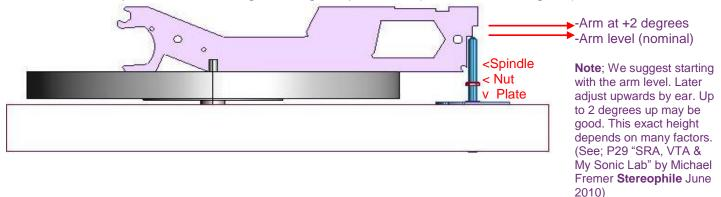
**Step 2;** Feed the bolt down to the boss on the clamping plate and loosely do up (but not tighten yet). NOTE; it needs to pass through the metal plate at the top and wood block underneath
