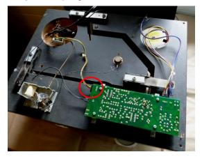
**Step 5;** Undo nut and remove the circuit board Cut the tonearm wires and discard the harness
