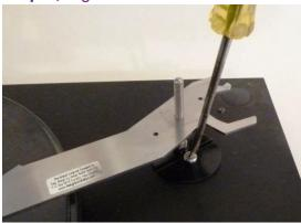
**Step 4;** Position mount using protractor. (Rotate to get in correct place).
