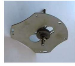
Hint: For the Classic model the locking nut can be above or below the boss. Above is more convenient but limits vertical height adjustment. Below gives slightly more space to adjust the arm.
