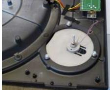
**Step 7**; Position the spindle sideways using protractor (& tighten screws)
