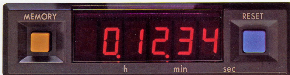
Tape accurate at all speeds, a microprocessor-controlled real-time counter features a Memory Rewind and L.E.D. display in hours, minutes and seconds.
