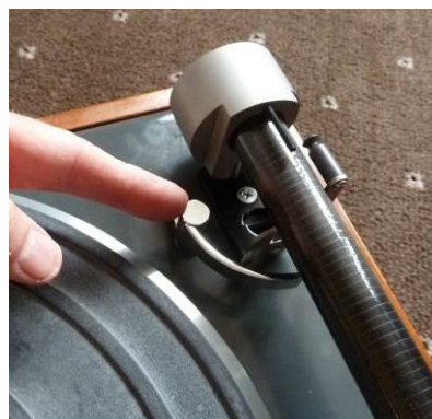
7; If using it, adjust Lenco arm lift and arm rest heights.
