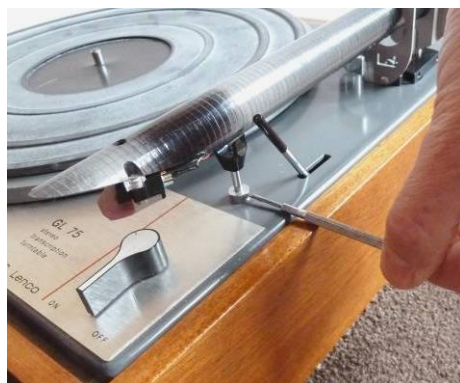
7; If using it, adjust Lenco arm lift and arm rest heights.
